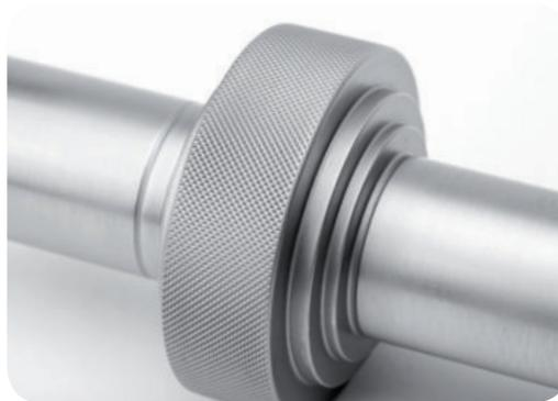
In this knurling technique it is not necessary to use beveled knurls, although it is always better so as to avoid premature breakage of the teeth angles. The bevels give strength to the edges of the knurls.
